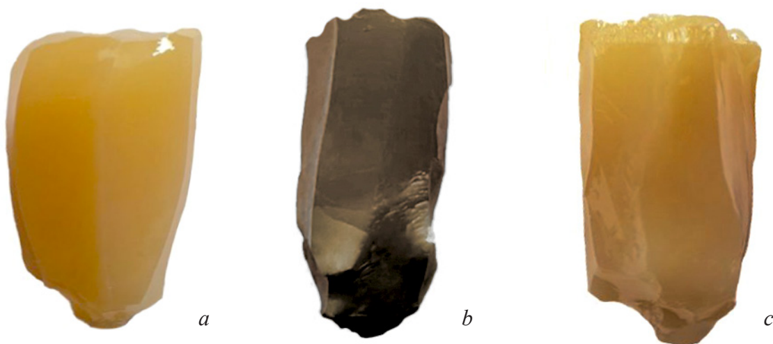
Figure 1. Appearance of 3.7SmSZ crystals (a) before and after (b) air and (c) vacuum annealing
