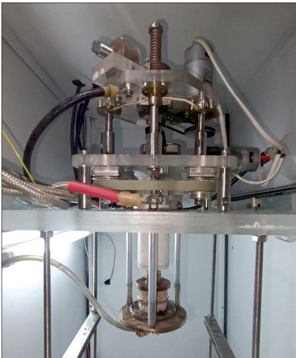
Figure 13. Electrode unit of electropulse plant for nanoparticle formation in liquid media
