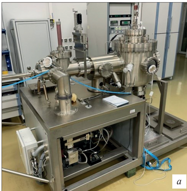
Figure 1. Nanostructure synthesis equipment: (a) Omicron ultrahigh-vacuum plant with four magnetron sputtering sources; (b) Suss Microtec MJB4 contact photolithography system
