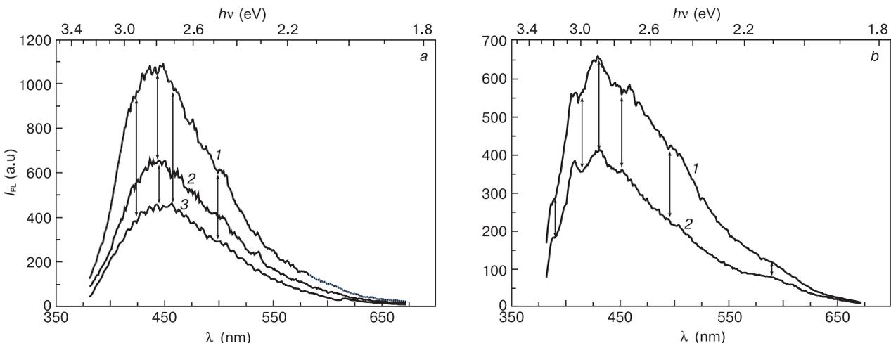
**Figure 2.**  $\lambda_{\text{ex}} = 355 \text{ nm}$  luminescence spectra of LGT crystals grown in different atmospheres for (a) 300 and (b) 95 K. a: (1) Ar; (2) Ar + 0.5 % O<sub>2</sub>; (3) Ar + 2 % O<sub>2</sub>; b: (1) Ar; (2) Ar + 2 % O<sub>2</sub>.
