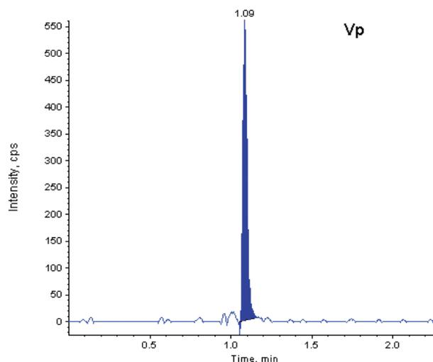
**Figure 3.** Typical multiple reaction monitoring chromatograms of verapamil.
