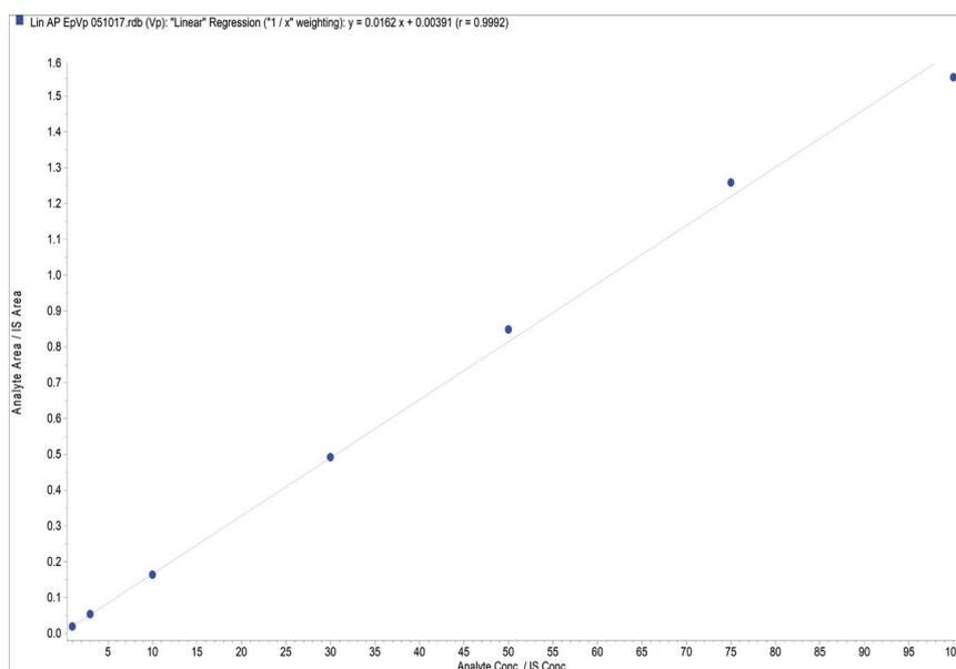
**Figure 4.** The calibration curve of verapamil hydrochloride in human plasma.
