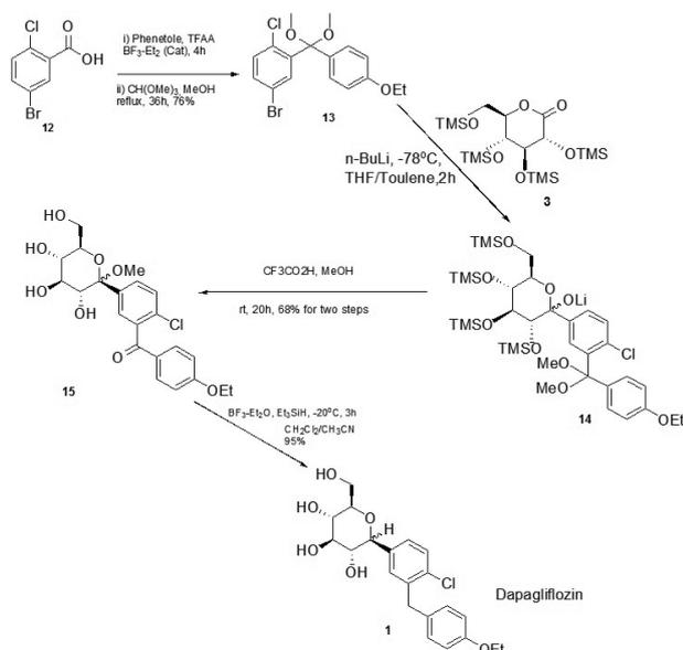
**Scheme 4.** Green route for the synthesis of dapagliflozin by Lin et al.
