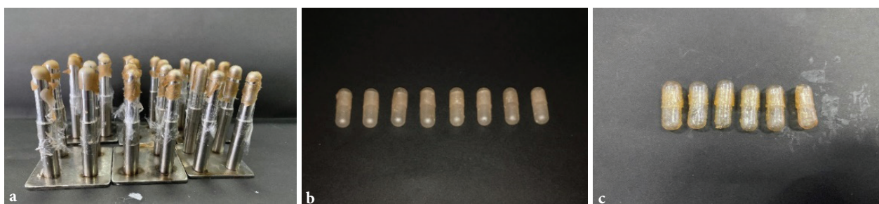
Figure 1. Capsule shell characteristics. a. Formula F1 (100%:0%) no capsule formed; b. Formula F2 (50%:50%) capsule rigid, strong, and smooth; and c. Formula F3 (0%:100%) capsule rigid, strong, and rough.
