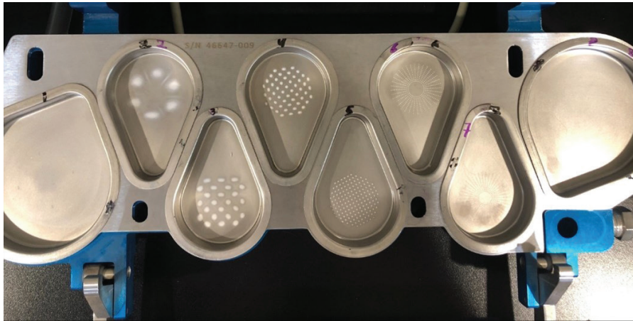
Figure 6. Image showing the deposition and distribution of erythromycin nanocrystals among next-generation impactor trays.
