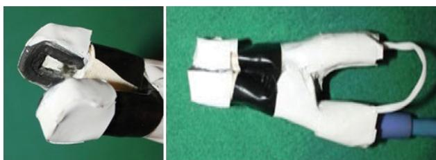
**Figure 2.** Custom-made sensor holder (Courtesy of Dr. Bargrizan).
