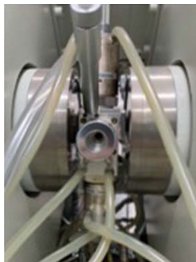
Figure 2. Irradiation aperture of the EPR-spectrometer.
