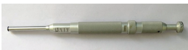
Figure 4. Implant driver with torque gauge (Absco Anchor LHD DT-S driver) consisting of resisting torque force ranging from 0.5 Kgf.Cm to 2.0 Kgf.Cm.
