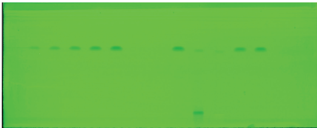
Figure 3. Chromatogram of sibutramine standard in concentrations from 0.250 µg/band to 1.250 µg/band and 5 dietary supplements.
