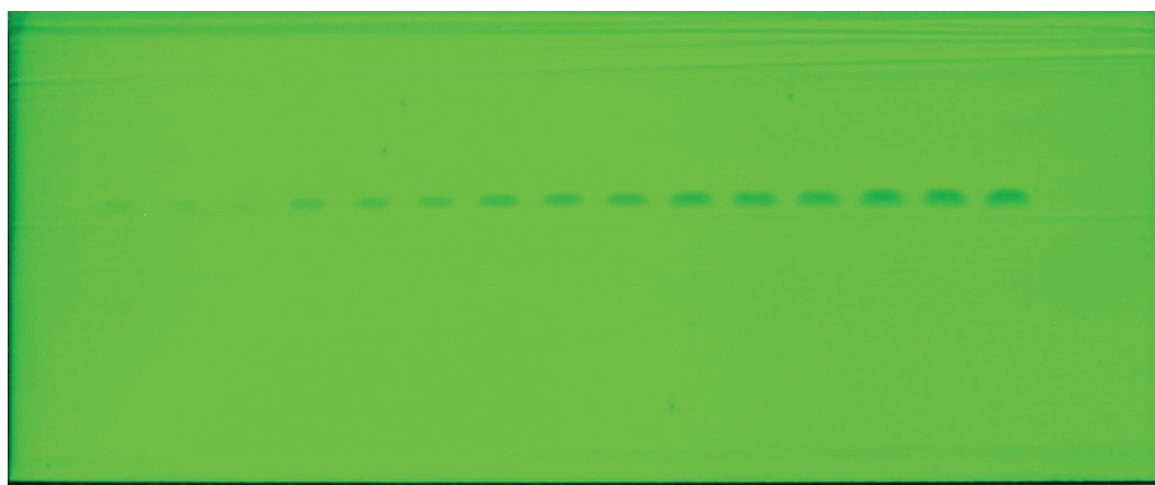
Figure 1. HPTLC chromatogram of sibutramine after derivatization with Dragendorff's reagent under 254 nm. Concentrations 250 ng/band, 500 ng/band, 750 ng/band, 1000 ng/band, and 1250 ng/band.
