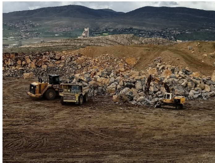
FIGURE 4. Secondary breaking process at New Cement Quarry (NCQ)
