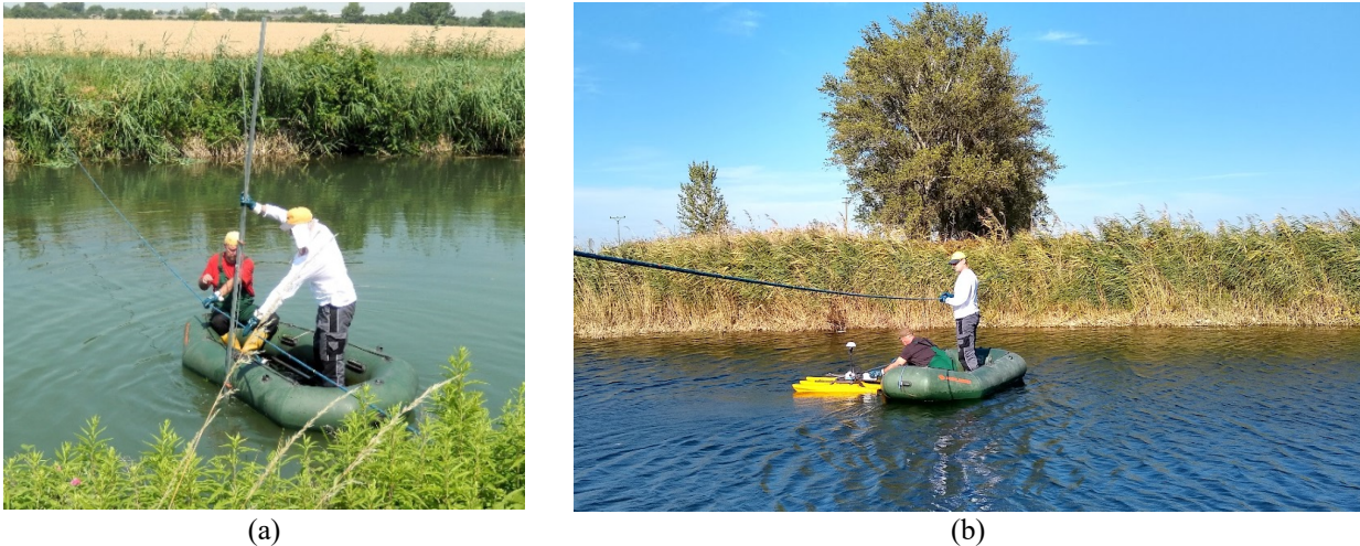
FIGURE 2. Field surveys on Gabčíkovo – Topolníky canal using manual method (a) and ADCP method (b). The ADCP device utilized for this study was the SonTek RiverSurveyor M9, a multi-frequency ADCP consisting of 4 beams operating at 1 MHz, 4 beams operating at 3 MHz, and vertical beam operating at 0.5 MHz. (Fig. 2b). Based on the current site conditions, a built-in algorithm, SmartPulseHD, automatically determines the appropriate acoustic pulse scheme at which the transducers emit and collect signals [5].
