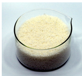
FIGURE 1. Synthetic wax F-T LC was added before foaming to bitumen 50/70 (fot. M.M. Iwański).
