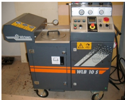
FIGURE 3. The WLB-10S asphalt foaming unit is characterised by the foaming properties of bitumen (fot. M.M. Iwański)
