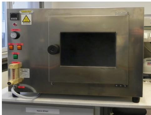
FIGURE 4. RTFOT asphalt ageing test apparatus (fot. M.M. Iwański)
