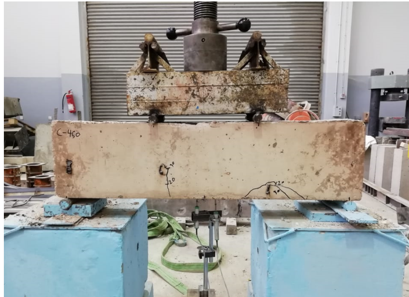
FIGURE 5. Two-Point load test setup
