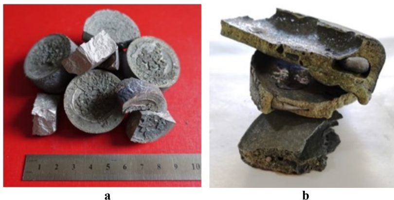
FIGURE 1. 1a- external view of the obtained ligature on the centrifugal machine; 1b- appearance of the ligature obtained in SHS reactor.
