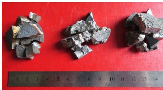
FIGURE 4. Appearance of complex carbide-forming ligatures obtained in the systems Fe- Mn-B -V, Fe-Mn-B W and Fe-Mn-B -Mo.
