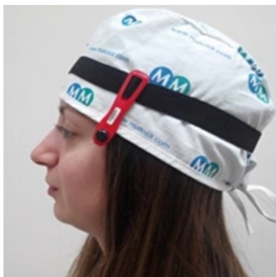
Fig. 1. Thermoluminescent dosimeter type EYE-D™ [24] and method of its attachment
